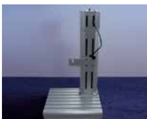
Bench with motorised column with automatic adjustment of stylus/part distance
